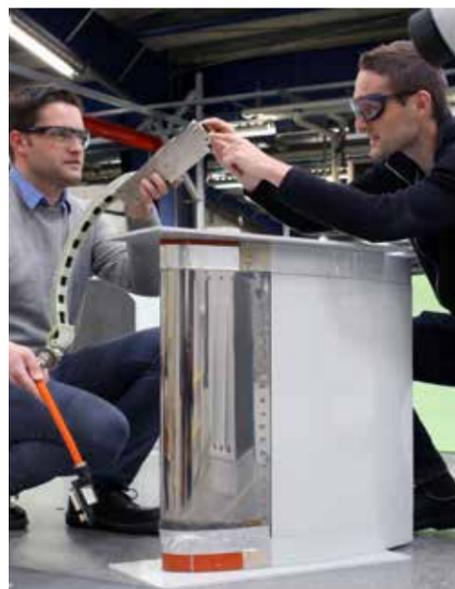
Slat with Electric Ice Protection System - demonstrator tested in icing tunnel to demonstrate TRL4 maturity level.
