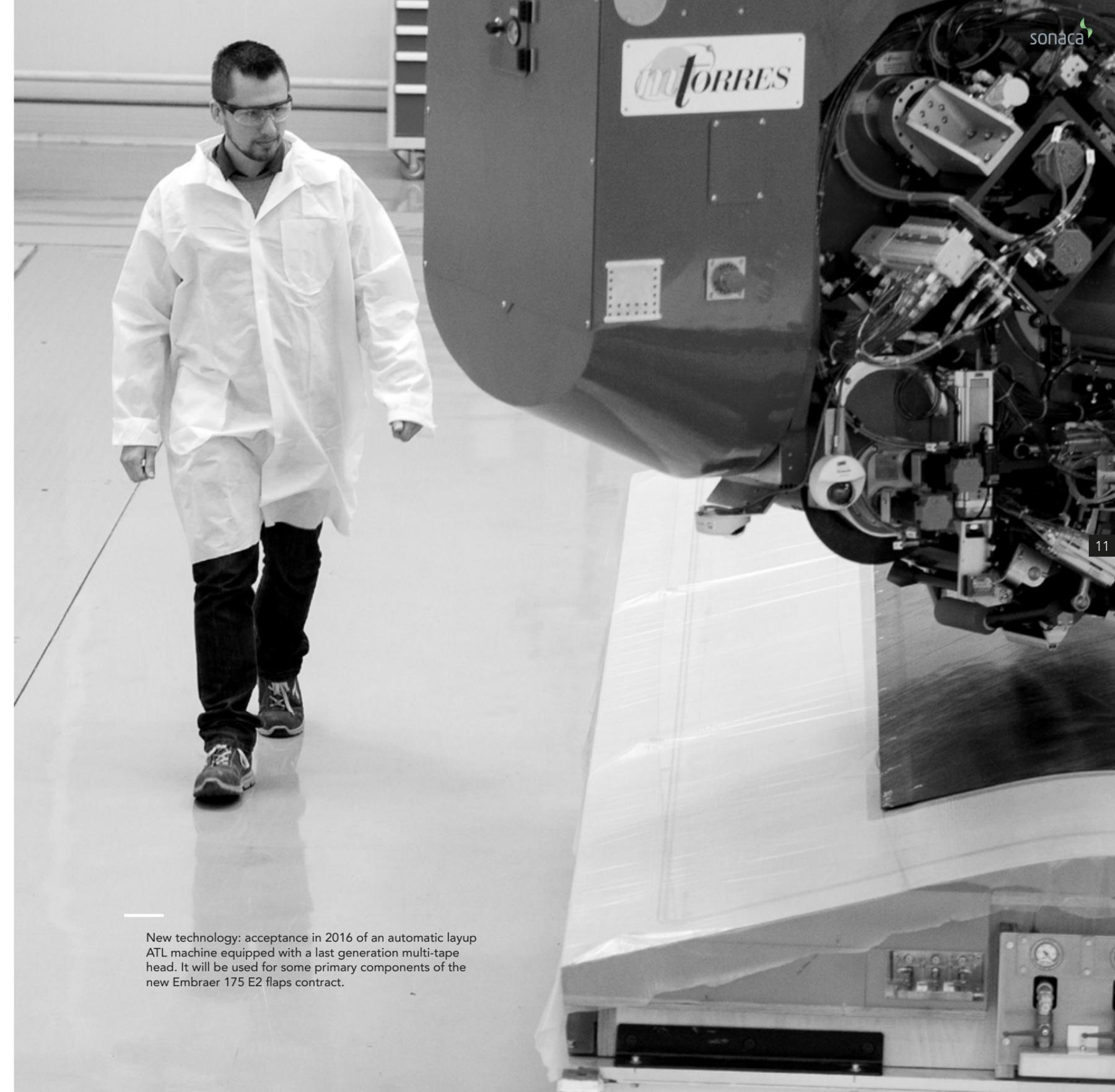
New technology: acceptance in 2016 of an automatic layup ATL machine equipped with a last generation multi-tape head. It will be used for some primary components of the new Embraer 175 E2 flaps contract.
