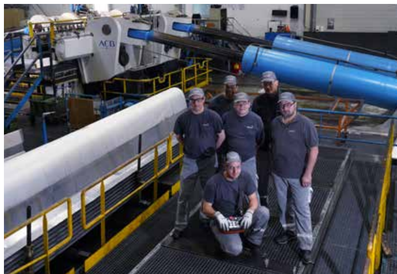
Sonaca Gosselies: stretching machine, 2500 tonnes - capable of stretching large wing leading edge part and fuselage panels.
