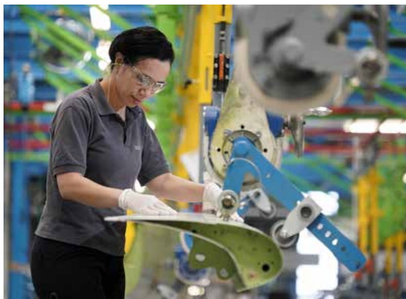
Sonaca Gosselies: complex slat assembly: A350. Over a thousand slats (all programs) leave the sonaca plants every month.
