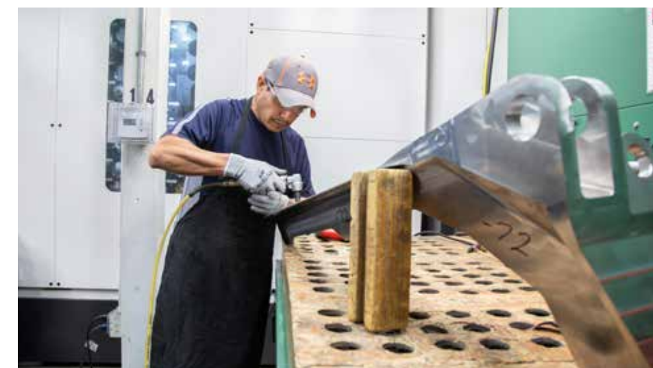
An LMI Aerospace employee in Washington (Mo) performs blending on a R3/R4 fitting.
