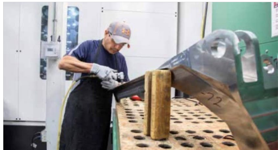
An LMI Aerospace employee in Washington (MO) performs blending on R3/R4 fitting
