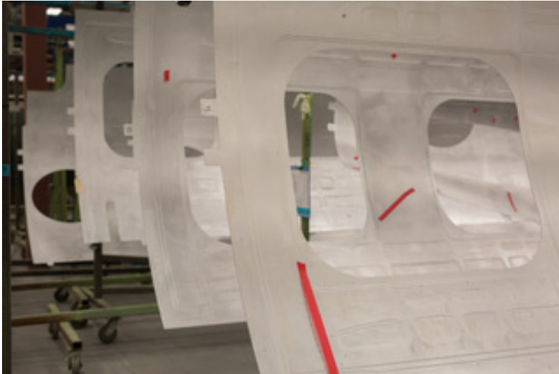
Skins of the bonded panels for our customer Gulfstream, made in Tulsa
