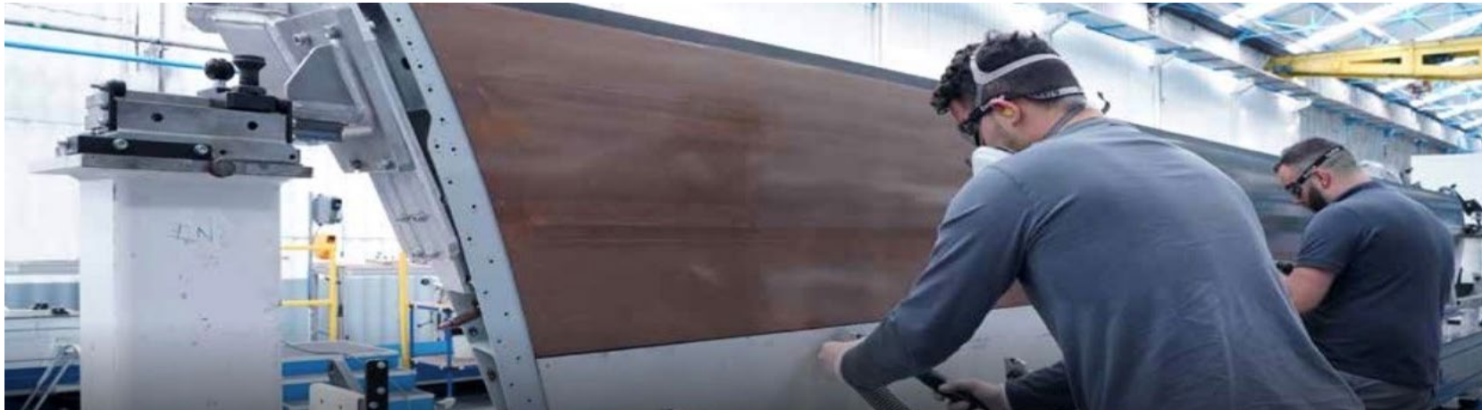
Sonaca Gosselies: outboard flap Embraer 190, highly complex composite/metallic assembly
