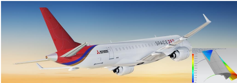
© by Mitsubishi Aircraft Corporation Conceptual studies and weight optimization of slats and flaps of Mitac Spacejet
