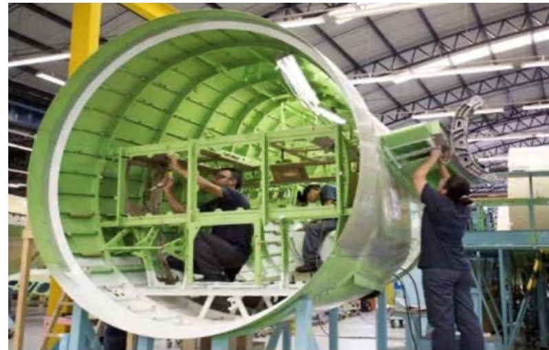
Sonaca Brasil: Legacy 500 rear fuselage complex assembly
