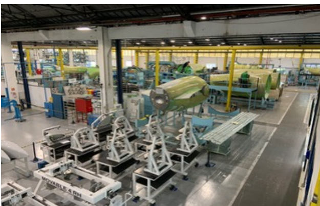
Complex assembly of rear fuselage in Sonaca Brasil
