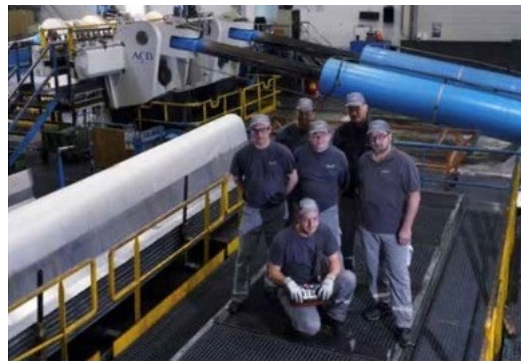
Sonaca Gosselies: stretching machine, 2500 tons – capable of stretching large wing leading edge parts and fuselage panels
