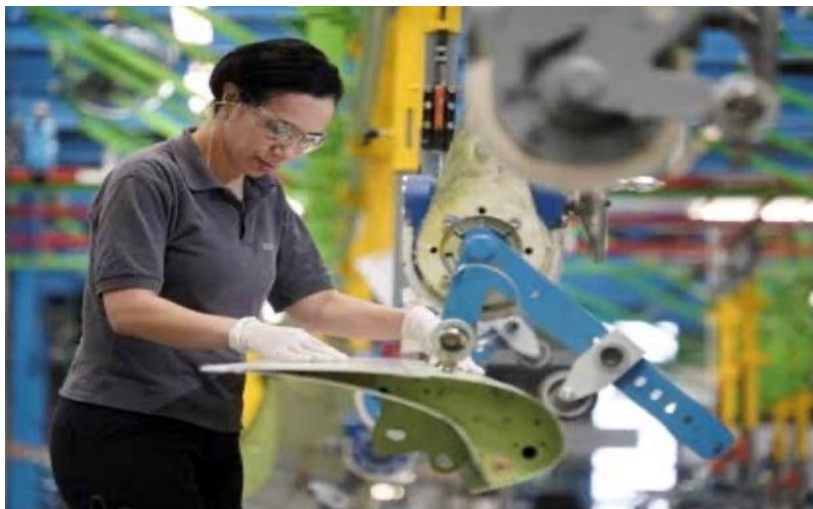
Sonaca Gosselies: A350 complex slat assembly Over one hundred slats (all programs) leave the Sonaca plants every month
