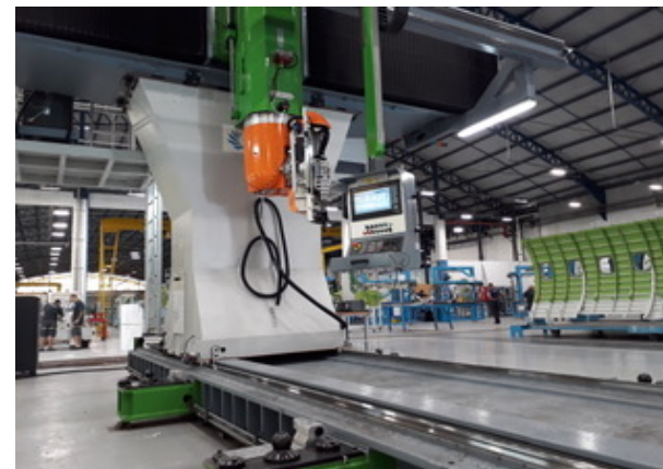
APIX machine for drilling E2 composite flaps (transfer from Sonaca Gosselies)
