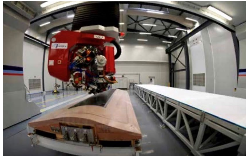
ATL (Automatic Tape Layer): Sonaca Gosselies composite department
