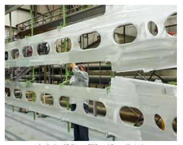
Anodization of Gulfstream G280 panel, Sonaca Montreal
