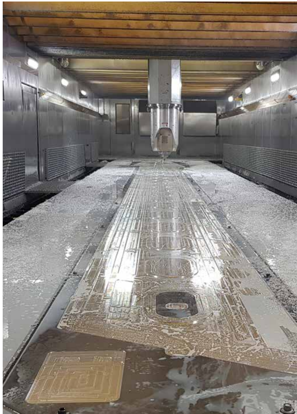
Sonaca Montreal is one of the only one-stop shops in the world to be able to produce skins and spars for wings and empennages 30 to 57 feet in length and up to 9 feet in width.
